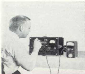
Calibrating the Type 761-A Vibration Meter with the Type 1557-A Vibration Calibrator.
